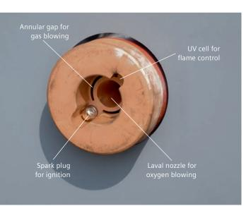
deviations or soiling of nozzles and is equipped with a UV cell for flame control during burning. In addition, the COB lance literally allows to keep an eye on the RH processes: With the integrated video camera, observation of the steel circulation and all events during treatment is possible.
