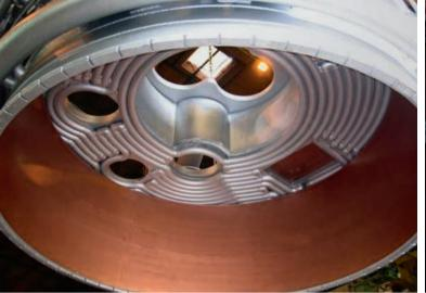
LF roof on the Siemens Metals Technologies workshop ready for delivery
