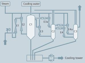
The vacuum pump systems necessary for vacuum degassing units are entirely designed and engineered by Siemens Metals Technologies process specialists. This ensures that the technical performance of each supplied pump system will meet the process and metallurgical requirements under all climatic conditions.
