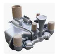
Figure 11 Outer wheel arch raw casting
