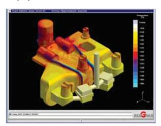
Figure 6 Simulation of temperature distribution
