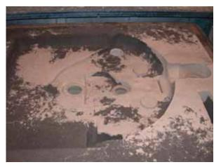
Figure 5 View at inner wheel arch cope mould
