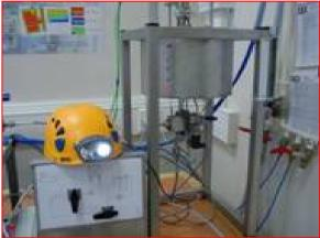
Helmet torch powered by Mg tank
