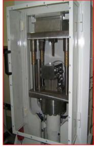
Equal-channel angular processing (ECAP)
