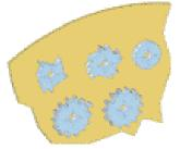
The PMMA is dissolved leaving a three dimensional metal micropart. Individual microparts can be separated from the base plate if desired.
