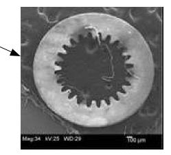
micrograph of MW sintered gear
