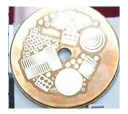
Nickel features electroplated on tool steel base
