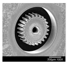
micrograph of gear mold
