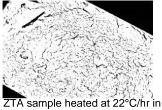
tube furnace with constant air flow
