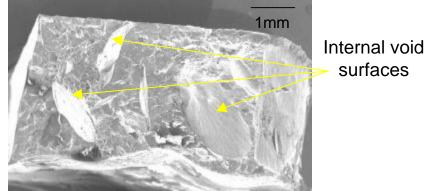
Alumina fracture surface
