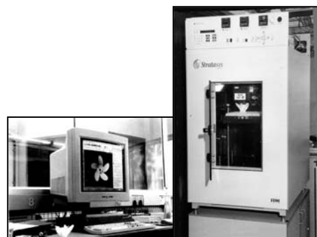
Fig. 3. Rapid Prototyping – from CAD model to part in hours
